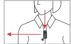
**"Surround"** – When SurfLink Remote Microphone 2 is placed horizontally (on its clip), it receives sound from all directions. This setting is useful for listening to multiple nearby speakers in quiet environments.
